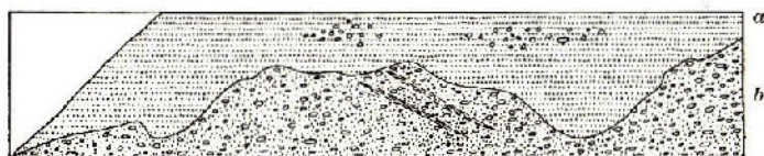
a , sand with irregularly distributed gravel. b , gravel with two lenses of clay.
